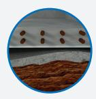
With PREPRUFE®, the membrane is fully sealed to the structural concrete and is unaffected by any ground settlement. The PREPRUFE® membrane remains fully bonded to the structure to resist hydrostatic pressure and avoid membrane stress.
