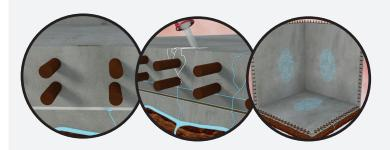
Conventional membranes are either unbonded or bonded to the substrate and normally covered with protective layers or screed separating them from the structure. When there is damage or a defect in the membrane, water can track between the membrane and the structural concrete looking for cracks or weakness in the concrete.
