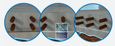
With PREPRUFE® membranes, the protection layer is eliminated and the membrane is bonded tightly to the structural concrete to prevent water penetration.
